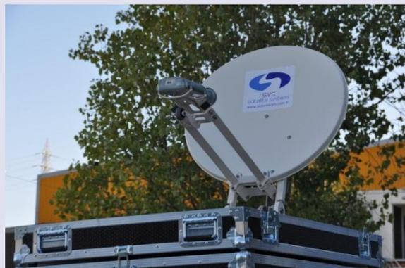
SVSATNM 78-Ka helps operator to find satellite with a user interface. Instead of motors, operator can find the desired satellite by adjusting to antenna reflector by looking to the computer screen. When satellite is found, the software warns you that it is "locked". The software also provides audio visual alarms.
